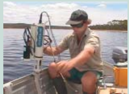
Figures 4, 5 and 6 (top to bottom): Analysing nutrient samples in a laboratory and sampling from the boat in Wilson Inlet with a Hydrolab instrument.
